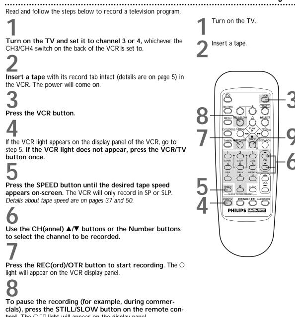
**trol.** The O II light will appear on the display panel. **To resume recording**, **press the STILL/SLOW button again.** The O light will appear on the display panel.
